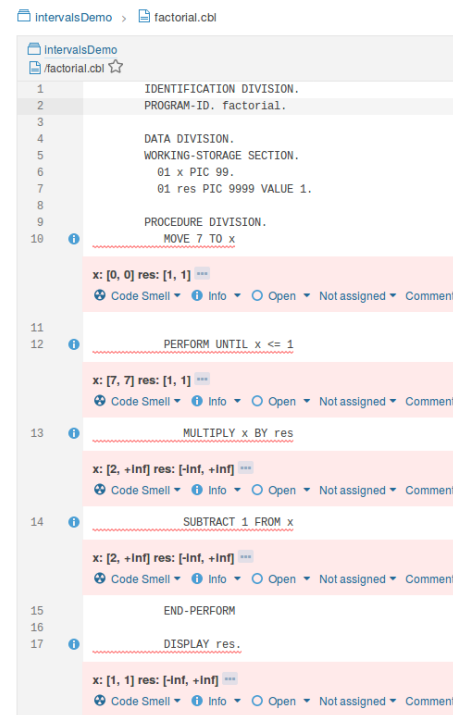
Figure 4. SonarQube view of interval analysis, where each issue represents intervals that are valid before the statement
